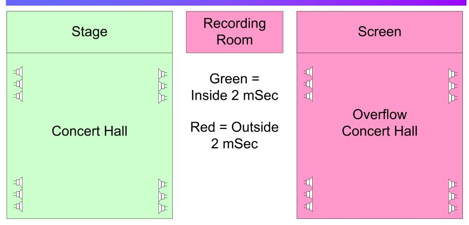
If Talkers use a normalize Sample Time the overflow Concert Hall can play all the data in-sync with the correct offsets given to it by the higher layer application
