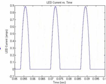
(c) Simulation of current through HB LEDs. Luminous intensity is proportional to current, causing lamp to flicker at the AC mains line frequency (shown periodic every 1/60 sec)
