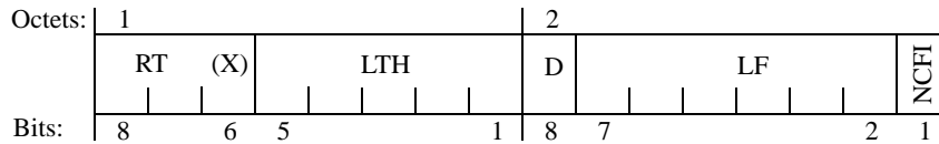
Figure 9-1—E-RIF Route Control (RC) field
