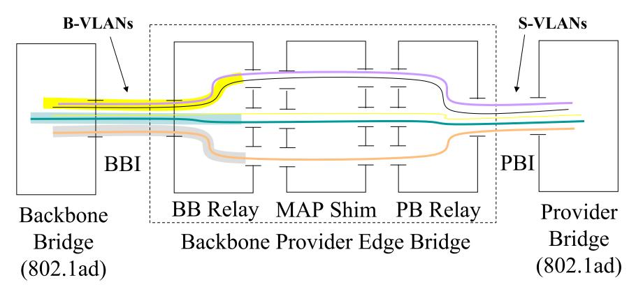
• MAP Shim performs encap/decap of frames to/from Provider Bridge Networks
