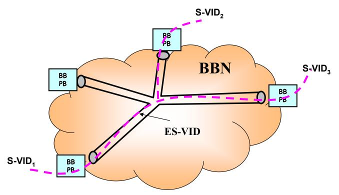
• Regardless of the ES-VID address size the map tables only have 4096 entries since only one ES-VID exists per S-VLAN and only 4096 S-VLANs exist per Provider Bridge.
