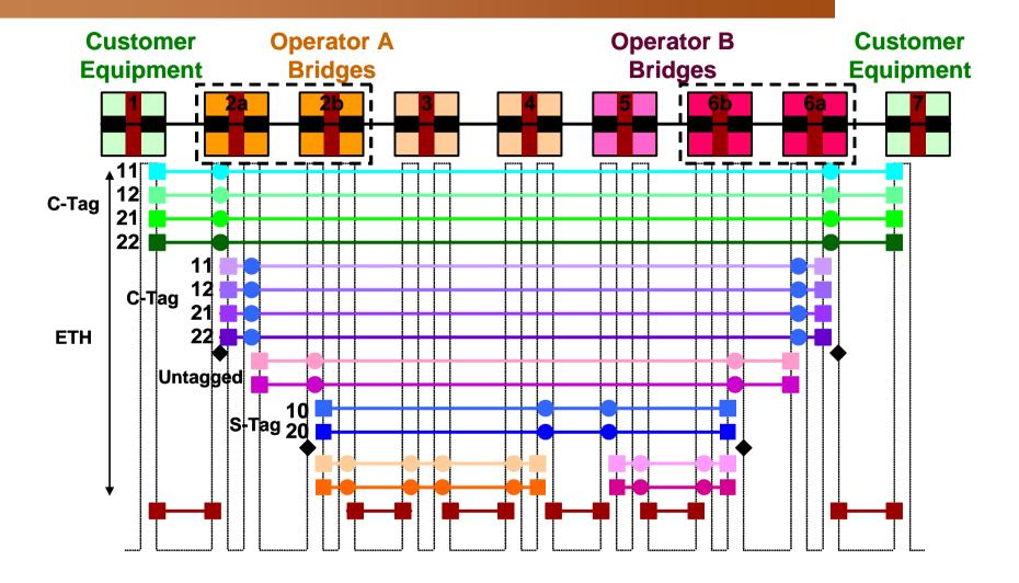
2a, 6a: peer customer L2CP protocols, multiplex user flow 2b, 6b: accommodate multiplexed user flow into a VLAN
