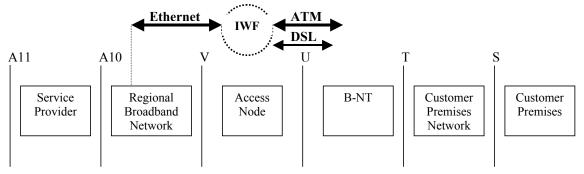
Figure 3 – ATM to Ethernet via Inter-Working Function
