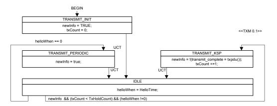
Figure 6 — Transmit state machine
