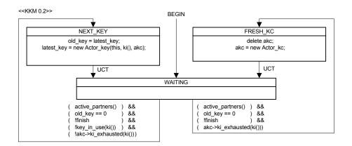
Figure 8 — Key Generation state machine
