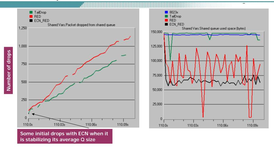
L2-CI can significantly reduce packet drops & reduce buffer requirements
