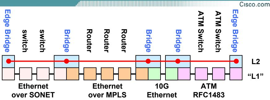
CFM: Standard Ethernet frames, distinguished from ordinary data frames only by destination MAC address and/or EtherType, and seen, relayed, and/or terminated by Provider Bridges.
