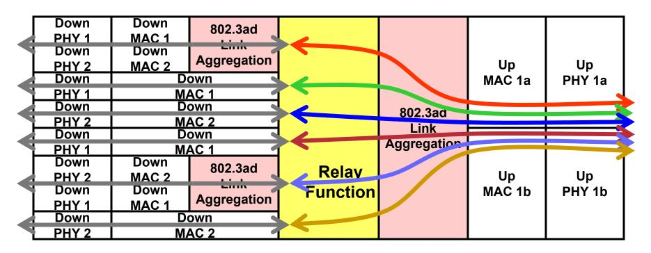
Rather like PVIDs, the Relay Function tags and untags frames on the Downlinks, and uses VLAN tags to multiplex the Uplink.
