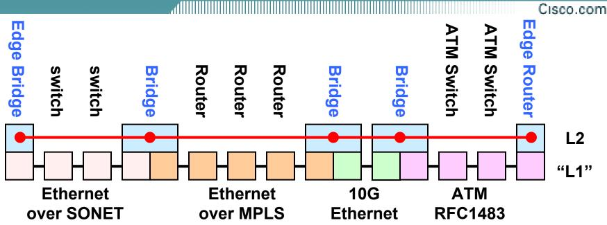
CM/OAM: Standard Ethernet frames, distinguished from ordinary data frames only by destination MAC address and/or EtherType, and seen, relayed, and/or terminated by Provider Bridges.
