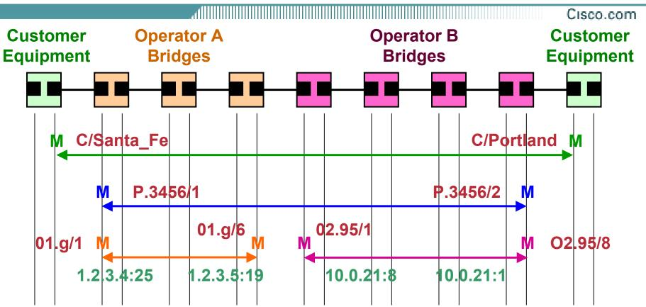
Operators assign MPIDs to specific hardware Interfaces (IP addr : ifIndex)
