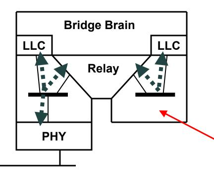
**Bridge transmits and** receives many frames, typically including IP bridge management traffic, and specifically for this example, E2E OAM packets, through a separate (virtual?) interface through the Relay Function.
