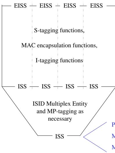
Customer data frames are constructed just as currently described in subclause 6.8 using the service-instance-with-encapsulated-ethernet tag (I-type).
