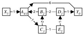
Figure 3—Packet looping in a loop-free network
