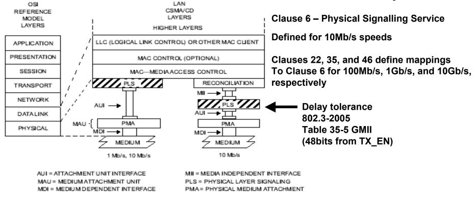
Figure 6–1—PLS service specification relationship to the ISO/IEC Open Systems Interconnection (OSI) reference model and the IEEE 802.3 CSMA/CD LAN model
