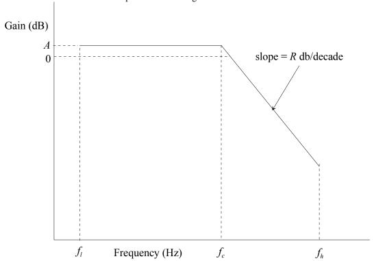
Figure 7. Example transfer requirement for filter, specific to application
