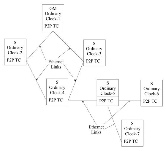
Figure 2. Illustration of AVB clock hierarchy
