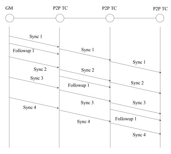
Note: The Followup messages corresponding to Sync2 and Sync3 are not shown to keep the diagram from being too cluttered.
