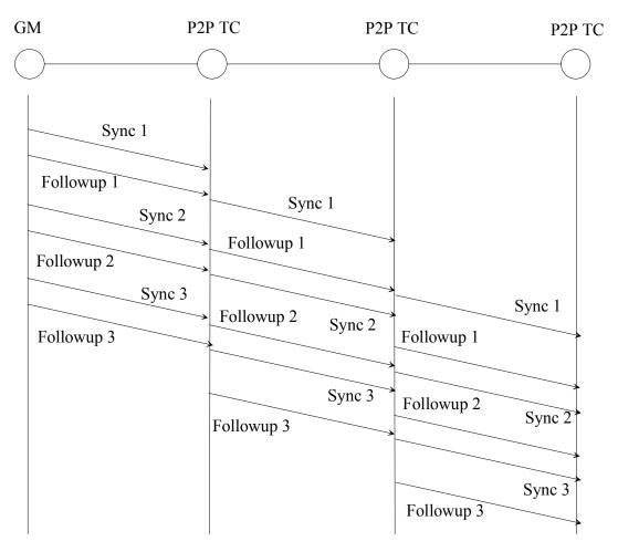
Figure 6. Sync and Followup sent with Sync held at P2P TC until corresponding Followup arrives. Followup processing time and sync interval are of the same order. Sync processing time is much less than Followup processing time.
