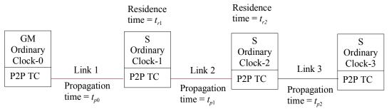
Figure 4. Illustration of accumulation of residence times and propagation times by P2P TCs
