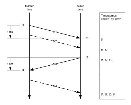
Figure 3. Basic synchronization message exchange (taken from[9])
