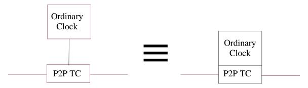
Figure 1. Illustration of implied single connection between an OC and the collocated P2P TC
