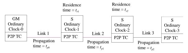
□The slave offset is computed when a Sync and corresponding Follow\_Up message are received by the slave, using Eq. (2-4) of [5]
