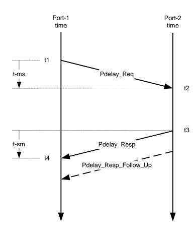
Propagation delay error = 0.5\*(t3 – t2) \* (frequency offset between the nodes)
