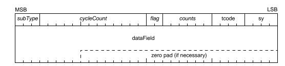
Figure C.4—Encapsulated IEEE 1394 frame payload
