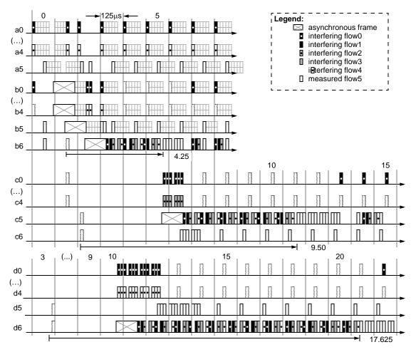
Figure F.16—Six source bunching; throttled-rate output-queue bridges
