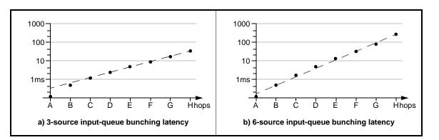
Figure F.8—Cumulative bunching latencies; input-queue bridge
