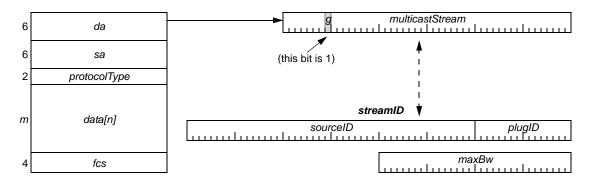
Figure 5.19—ClassA frame format and associated data
