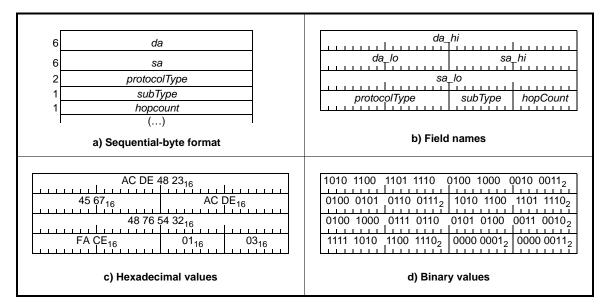
Figure 3.5—Illustration of fairness-frame structure
