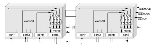
Figure 11.3—Reshaped bridge-traffic topology, with bunching control
