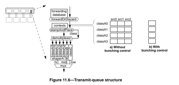
The intent of per-class shapers is to avoid priority inversions, wherein higher-class frames are delayed by the presence of concurrent lower-class traffic. Independent per-class shapers and queues allow enqueued higher-class and lower-class frames to be forwarded independently, thus avoiding priority inversions within queues.
