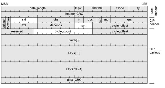
Figure C.7—Isochronous 1394 CIP packet format
