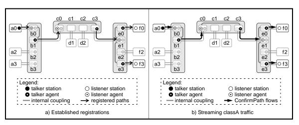
Figure 5.14—Streaming data over registered paths
