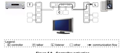
Figure 5.8—Controller activation
