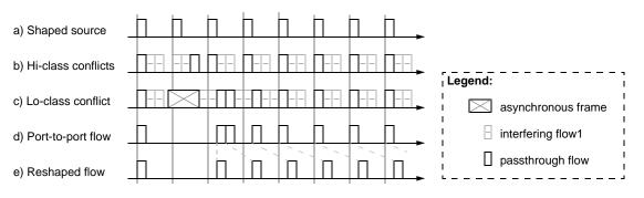
Figure 11.4—Reshaped bridge-traffic timing
