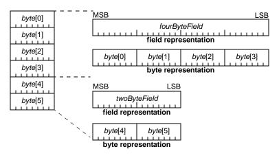
Figure 3.4—Multibyte field illustrations
