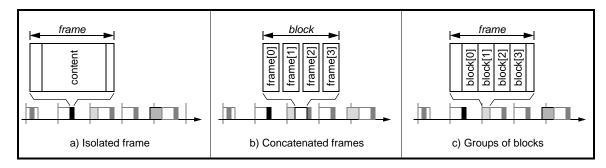
Figure 5.17—Content framing methods
