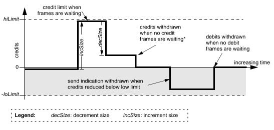
Figure 10.9—Credit adjustments over time
