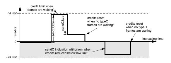
Figure 11.9—Pacer credit adjustments over time
