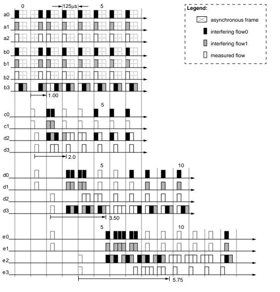
Figure F.18—Three-source bunching; throttled-rate output-queue bridges
