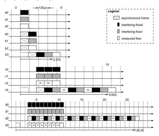
Figure F.4—Three-source bunching timing; input-queue bridges
