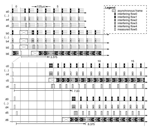
Figure F.10—Six source bunching; output-queue bridges
