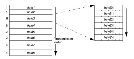
Figure 3.3—Byte sequential field format illustrations
