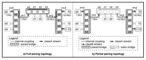
Figure 10.1—Topology-dependent pacing delays
