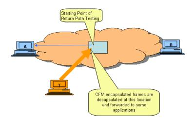
Figure 40-2—Return Path Testing
