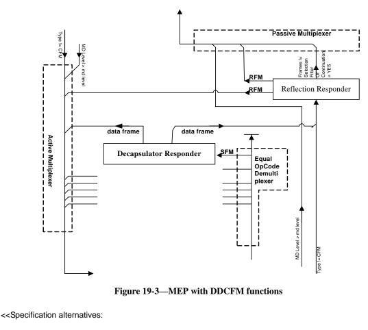
1) Instead of providing the Reflection functionality within a CFM shim, as shown above, that could be done within the Forwarding Process of the bridge's MAC Relay Entity, using the Filtering Database (possibly extended) to provide the necessary controls. That approach might be a natural extension of the existing
