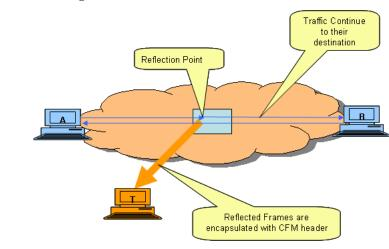
Figure 40-1—Forward Path Test
