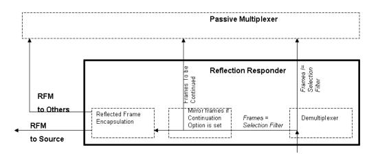
Figure 40-4—Detailed Functions of Reflection Responder
