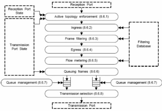
Figure 8-9—Forwarding Process functions
