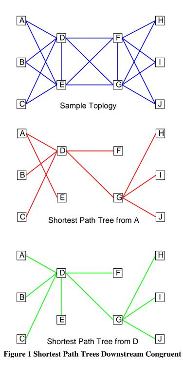
In Figure 1 we have a sample topology where there are two shortest path trees shown rooted at A and D. It is assumed all links have equal weight in this figure.
