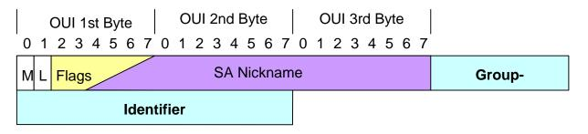
Figure 5: Multicast B-DMAC Encoding
