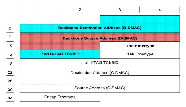
Figure 3 802.1 PBB Header
