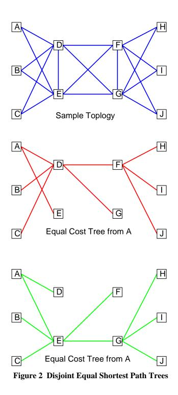
For those familiar with Equal Cost Multiple Path (ECMP) in IP will note there are differences between the ECMT of Ethernet bridging. ECMP selection is performed Hop by Hop. ECMT is performed on a per logical VLAN basis the path is determined by the tree chosen.
