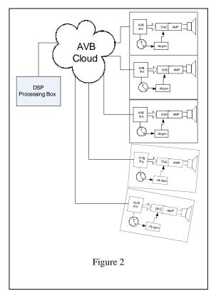
Line arrays are designed to produce sound in a large area using carefully designed speaker pattern overlap often referred to as beam engineering. Modern beam engineering uses a combination of physical placement and digital signal processing. Uncertainty in the phase relationship of the word clocks driving the digital to analog converters is a known source of system degradation. Accuracy of the AVB RTC will have a direct impact on the phase accuracy of the word clocks.
