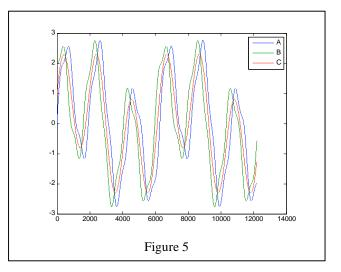
In this example it is evident that the shape of waveform C is different from that of the waveform at A or B. The phase difference in the word clocks has resulted in what we call destructive interference. A reasonable way to quantify the difference in shape of A and C
