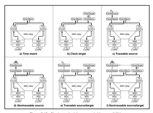
Figure 5.15—Clock-attached time-aware bridge possibilities
