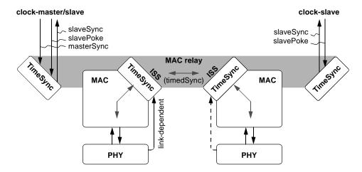
Figure 6.1—MAC-relay interface model
