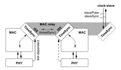
Figure 6.11—Clock-slave interface model
