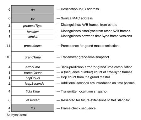
Figure 9.3—timeSync frame format
