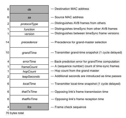
Figure 7.5—timeSync frame format
