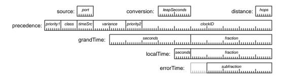
Figure 6.2—MAC-relay frame components
