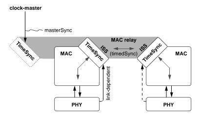
Figure 6.10—Clock-master interface model
