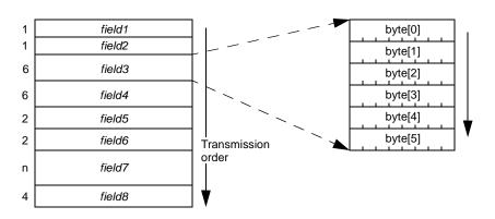
Figure 3.2—Byte sequential field format illustrations
