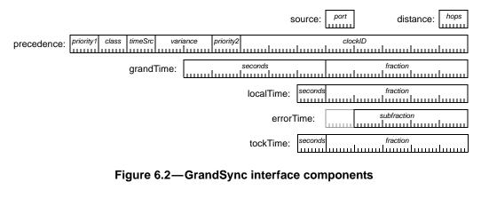
Information exchanged with the GrandSync entity includes a source-*port* identifier, *hops&precedence* information for grand-master selection, a globally synchronized *grandTime*, neighbor-syntonized *localTime*, and a cumulative *errorTime*, as illustrated in Figure 6.2. A clock-slave end-point can filter the sum of *grandTime* and *errorTime* values, thereby yielding its image of the globally synchronized *grandTime* value.
