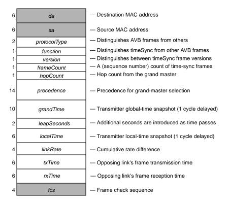
Figure 6.2—timeSync frame format
