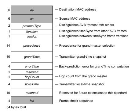
Figure 10.3—timeSyncPon frame format
