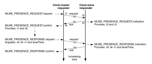
Figure 9.3—802.11v time-synchronization interfaces
