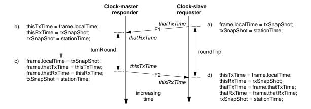
Figure 8.3—Link-delay compensation
