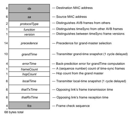
Figure 8.4—timeSyncDuplex frame format
