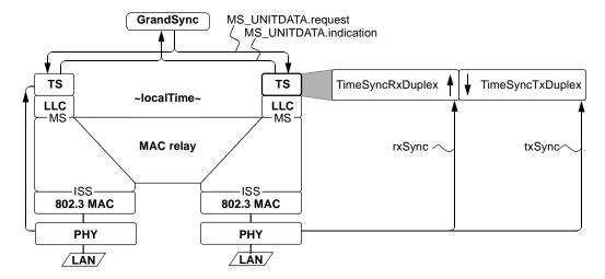
Figure 8.1—Duplex-link interface model
