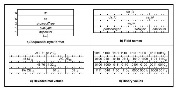
Figure 3.4—Illustration of fairness-frame structure
