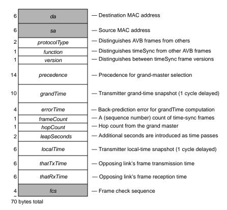
Figure 7.3—timeSync frame format
