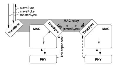
Figure 6.10—Clock-master interface model
