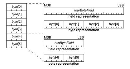
Figure 3.3—Multibyte field illustrations
