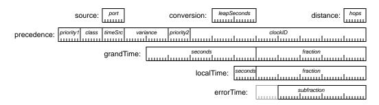
Figure 6.2—MAC-relay frame components
