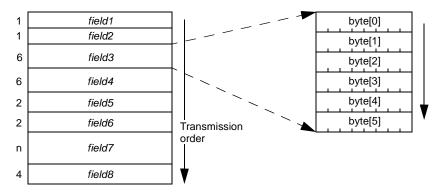
Figure 3.2—Byte sequential field format illustrations
