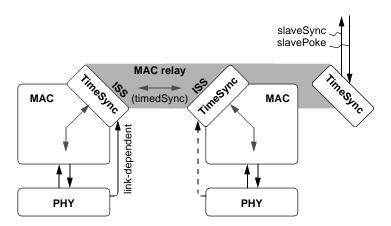
Figure 6.11—Clock-slave interface model
