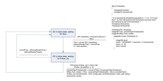
Figure 2-5. State machine, and corresponding C code, for receipt of Sync and Follow\_Up by an ordinary clock
