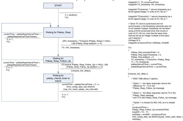
Figure 2-2. State machine, and corresponding C code, for Pdelay requestor P2P TC port
