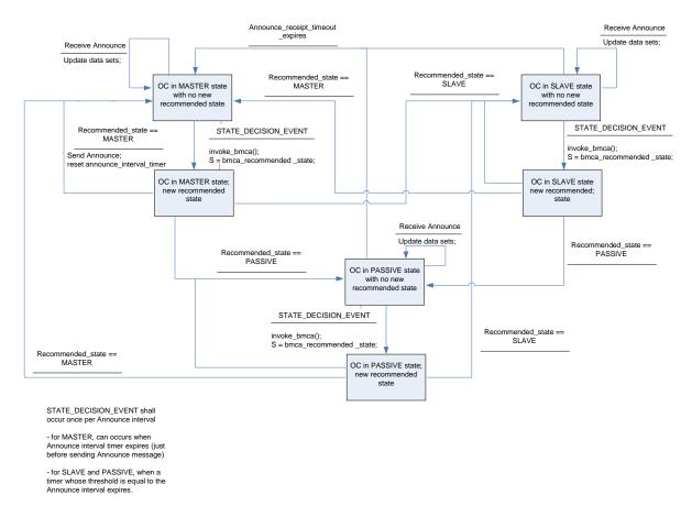
Figure 2-7. Simplified state machine for receiving and sending of Announce by an ordinary clock
