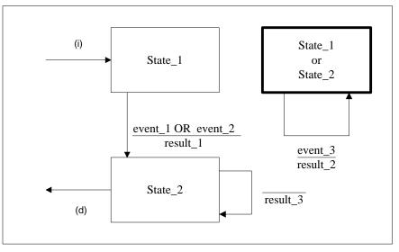
Figure 1 : Mealy state transition diagram
