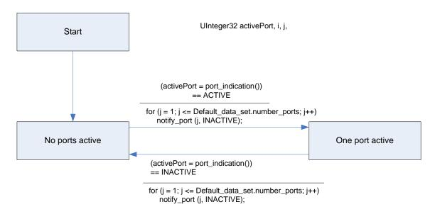
Figure 2-3. State machine, and corresponding C code, for a peer-to-peer transparent clock node
