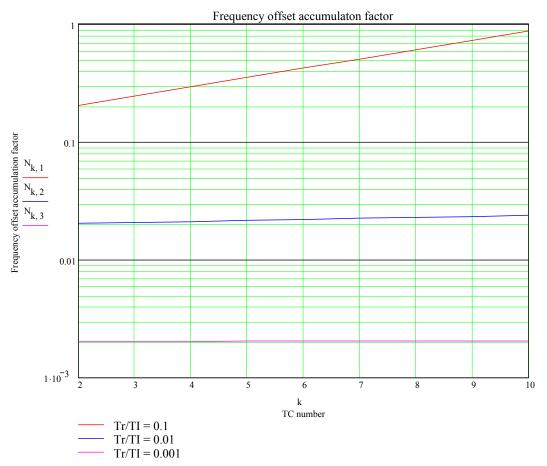
**Figure 1**. Factor by which frequency offset amplitude, due to applied sinusoidal perturbation, accumulates, as a function of TC number, for several ratios  $T_r/T_L$
