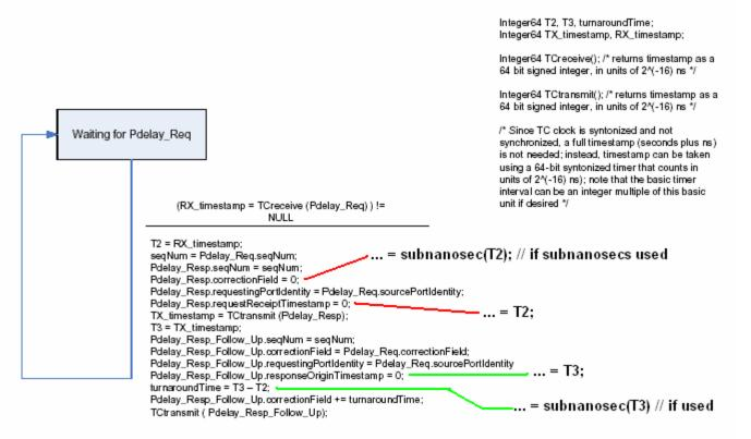
Figure 2-1. State machine, and corresponding C code, for Pdelay responder P2P TC port
