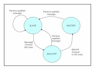
Figure 7-9. Clock Entity state diagram.
