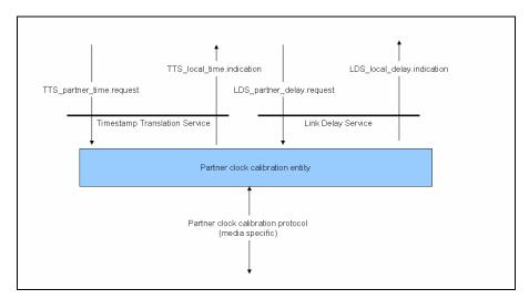
Figure 7-4. TTS and LDS interfaces.
