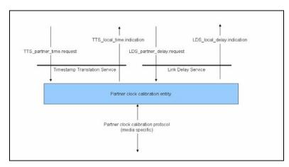
Figure 7-4. TTS and LDS interfaces.
