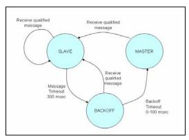
Figure 7-10. Global clock entity state diagram.
