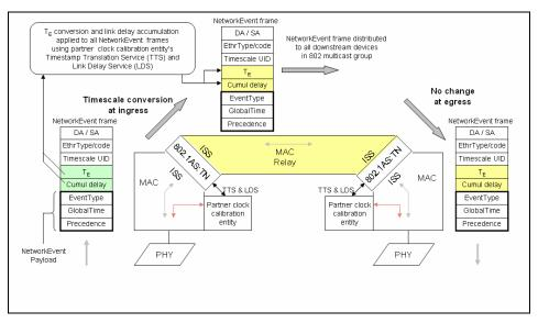
Figure 7-9. Network event frame forwarding model in 802.1D bridging environment.
