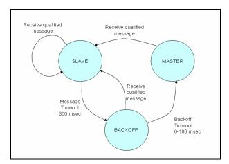
Figure 7-10. Global clock entity state diagram.
