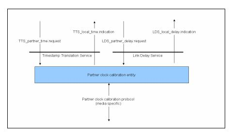
Figure 7-4. TTS and LDS interfaces.
