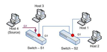
A periodic "garbage collector" mechanism shall check the adequacy between subscriptions and switch's port state, and block any port which is no more on a given multicast A/V traffic path.
