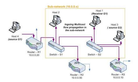
This request opens the sub-network to the requested source flow through the marked port of the IGMP router
