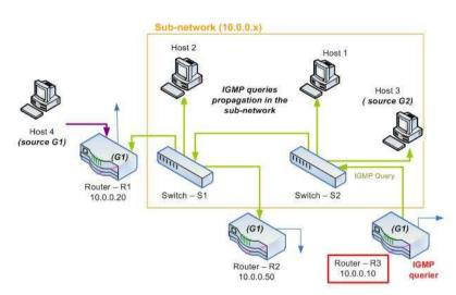
•To reduce IGMP traffic. a single IGMP querier is elected.
