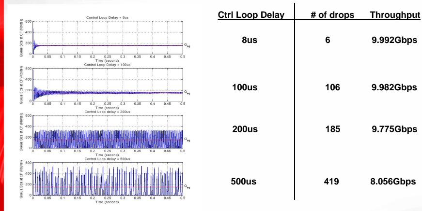
Mild throughput degradation and increase in frame drops as control loop delay increases. Derivative weight 'w' is kept at 2 in all of these experiments. At 200us and above, underutilization begins to occur.
