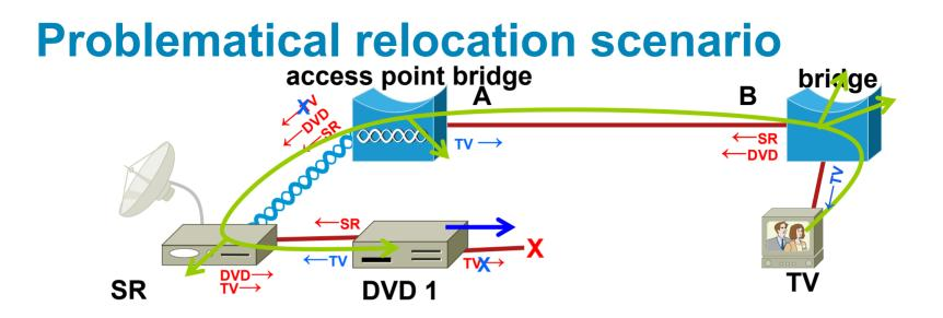
Applying the current solution, bridge B does not send a TCN, and instead, the TV sends some broadcasts and/or multicasts.
