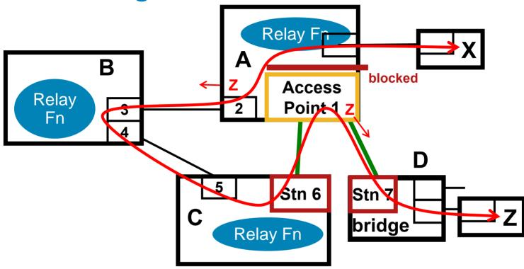
For example, in this case, the bridge part of A learns that station Z is on port 2, while the access point part of A learns that Z is on the wireless link to D.
