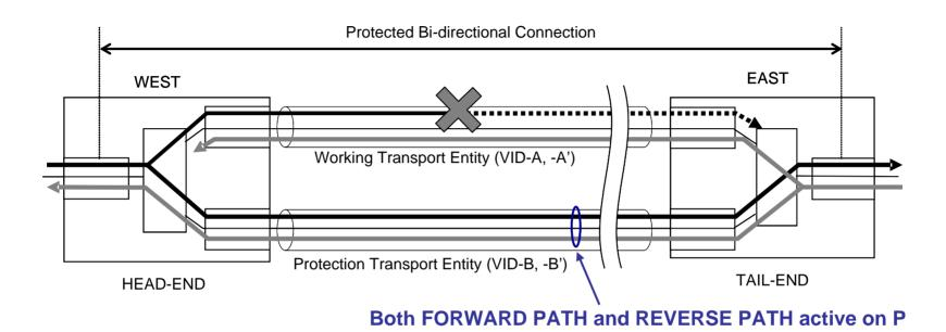
Note: In bi-directional switching, although both ends are performing both the Bridge (head-end) and the Selector (tail-end) functions, typically the term "tail-end" still refers to the end initiating the protection Switch and "head-end" still refers to the other end.
