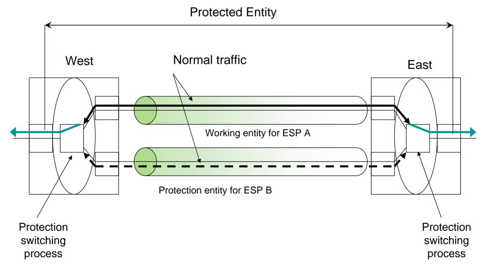
Normal traffic is transmitted via the working entity. There is no extra traffic on ESP B
