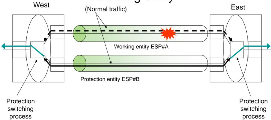
A protection switching event has occurred, due to signal fail condition on the working entity. At the source node the normal traffic is forwarded to the protection entity ESP#B. At the sink node, the normal traffic is received from the protection entity.
