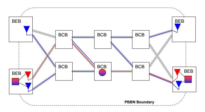
Scope of paths (CO) and BVLANs (CL) is defined by the PBBN boundary. CFM performed within this boundary is secure.
