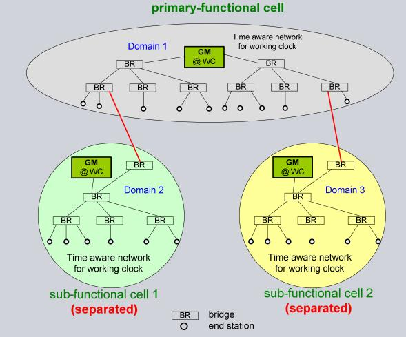
The working clock islands are still separated! Avoid auto merging of independent sub-functional cell to on sync domain!
