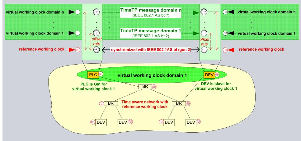
PLC: Programmable logic controller DEV: Device e.g. sensor or actuator BR: Bridge
