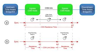
Fig. 6: IEEE 802.AS Sync Message Propagation over CSN
