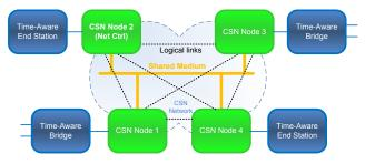
Fig. 5: Example of CSN Backbone in an AVB LAN
