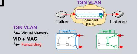
\*) Forwarding based on setup paths using MAC + VID – an example using this mechanism is SPB-V
