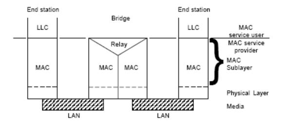
Figure 4—Internal organization of the MAC sublayer with bridging IEEE Std 802-2001 Overview and Architecture
