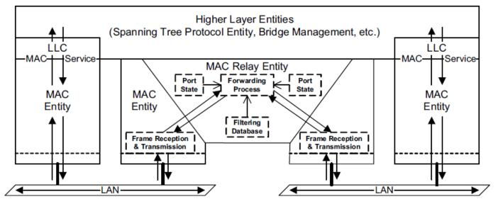
Figure 8-11—Logical points of attachment of the Higher Layer and Relay Entities
