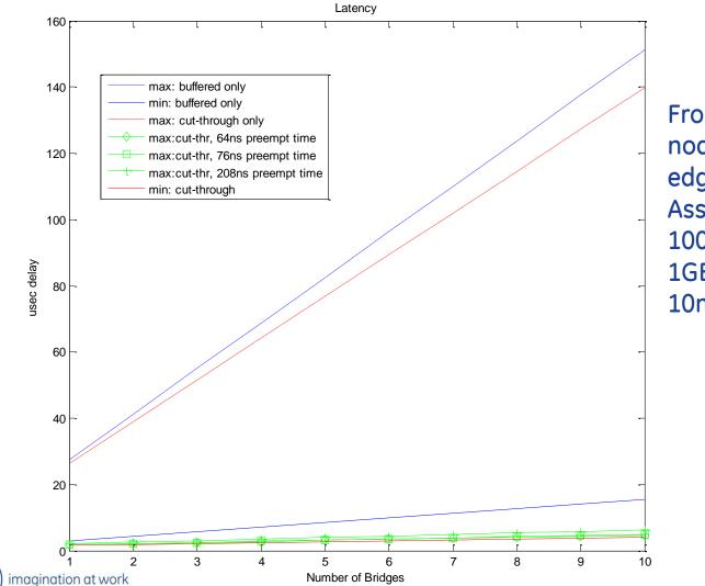
From xmit bit on edge node to last recv bit on edge node. Assumes: 100 byte packet 1GE 10m cable
