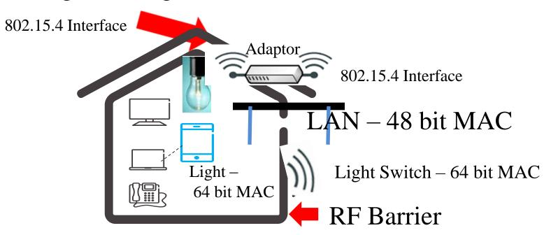
64 bit MAC to 48 bit MAC Adaptor/Bridge is the only solution to provide switch control to the lights in this scenario
