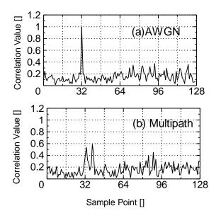
Fig. 7 Waveform of Correlation Output for [OFDM preamble + OFDM Data Symbol]
