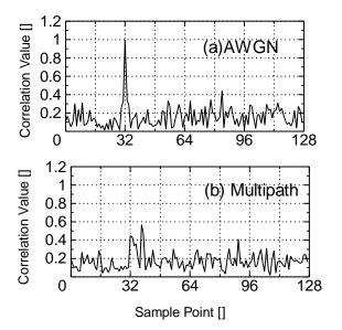
Fig. 6 Waveform of Correlation Output for [PN preamble + OFDM Data Symbol]
