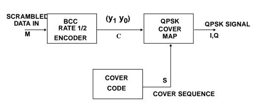
Figure 12. PBCC Modulator Scheme
