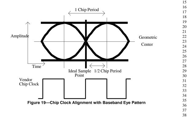
Using the aligned chip clock, 1000 samples of the I and Q baseband outputs from the reference receiver are captured. The vector error magnitudes shall be calculated as follows:
