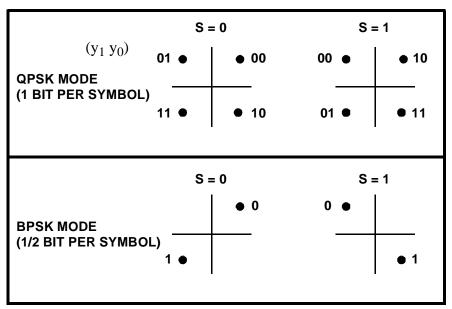
Figure 14. Cover Code Mapping
