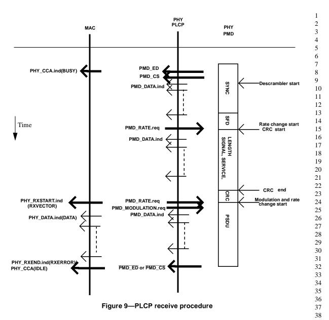
code lock prior to correct reception of the PLCP header. The PMD primitives PMD\_SQ and PMD\_RSSI are issued to update the RSSI and SQ parameters reported to the MAC.
