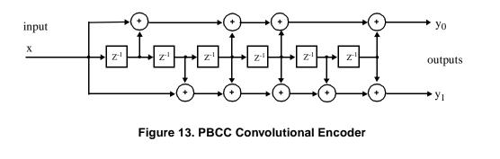
The output of the binary convolutional code described in above is mapped to a constellation using one of two1possible rates. The 5.5 Mbps rate uses BPSK and the 11 Mbps rate uses QPSK. In QPSK mode each pair of2output bits from the binary convolutional code is used to produce one symbol, while in BPSK mode each3pair of bits from the BCC is taken serially and used to produce two BPSK symbols. This yields a throughput4of one bit per symbol in QPSK mode and one-half a bit per symbol in BPSK mode.5
