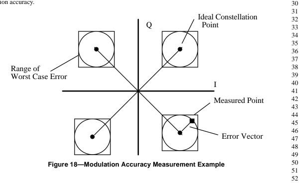
Error vector measurement requires a reference receiver capable of carrier lock. All measurements shall be made under carrier lock conditions. The distortion induced in the constellation by the reference receiver 54
